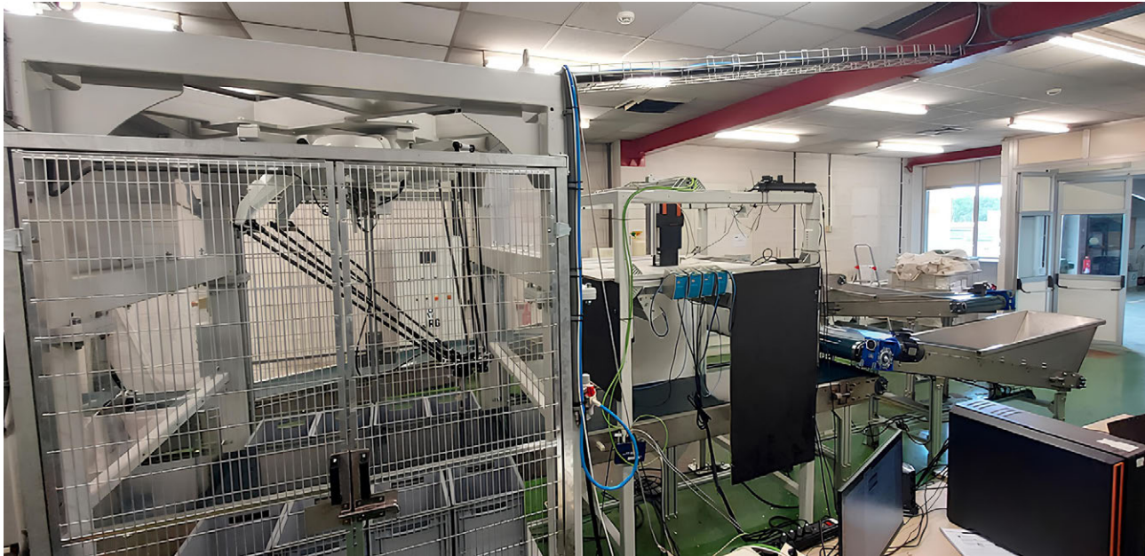
Robotic test line for classification and subsequent sorting of C&DW fragments (Tecnalia).
