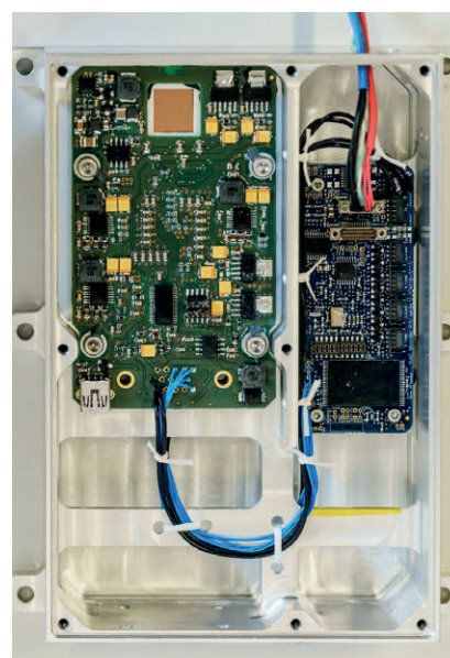
A flying part of the RISEPix monitor. The control module is on the right, detector modules are on the left – only the upper one is visible here.
