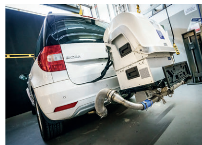
Portable emissions measuring system in live operation at CVSM Rostoky
